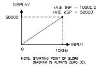
If the rate application is to display a specific display unit, it is only necessary to know the number of pulses per desired display unit/s (feet, revolutions, etc.) and in the desired time format, per second (1), per minute (60), or per hour (3600) to scale the rate display. Use the following formula to calculate the rate input value:
